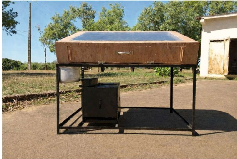
Figure 3 : Solar ice-making machine built in Antsiranana
