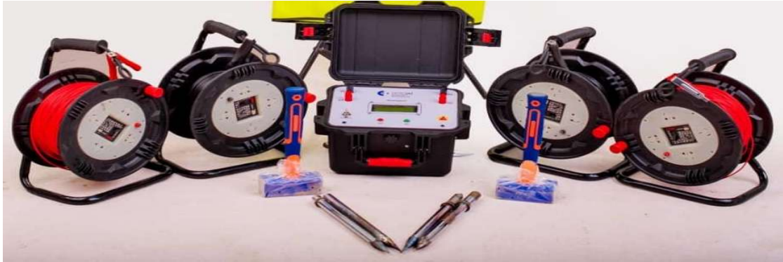
Fig. 2: Resistivity equipment for subsurface investigation (Field array setup showing terrameter hub, cable reels, hammers, and grounding electrodes)
