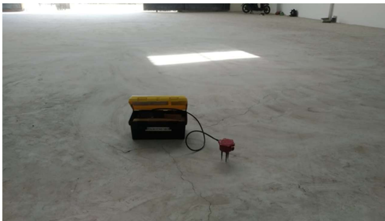
Fig. 1 Microtremor data acquisition inside a building with cement-cast flooring
