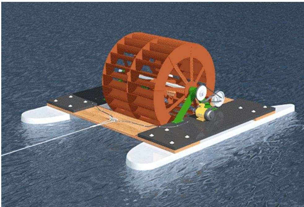
Figure 4 : Illustration d'Hydrolienne Flottante (source : Tech Briefs TEChBRIEFS)
