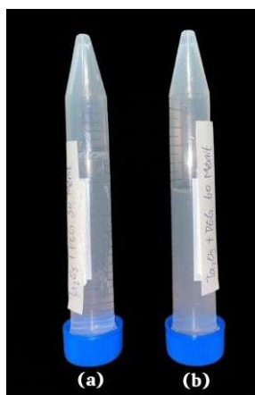
Figure 2. Colloidal tantalum oxide nanoparticles in a polyethylene glycol (PEG) medium with different synthesis times: (a) 30 minutes and (b) 60 minutes
