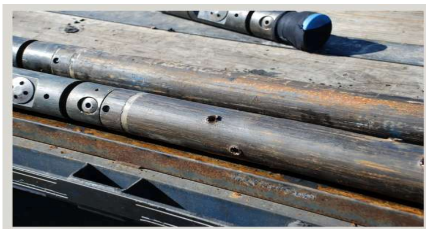
Figure 7: A perforating gun, a key tool in creating wellbore conduits for hydraulic fracturing, highlighting (After USGS 2016)
