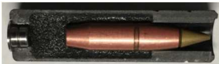
Figure 7. Cross-section of a 6.8 mm CT bullet cartridge
