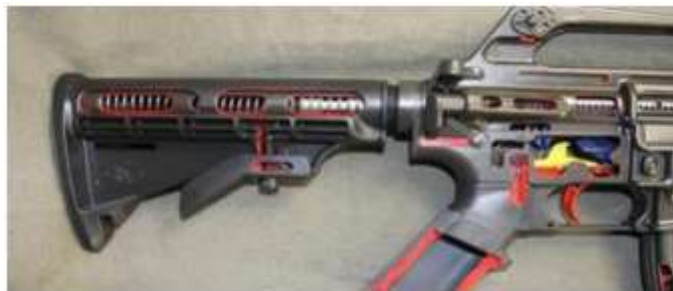
Figure 11. 5.56 mm Caliber M16A1 Assault Rifle whose recoil mechanism is in the stock.
