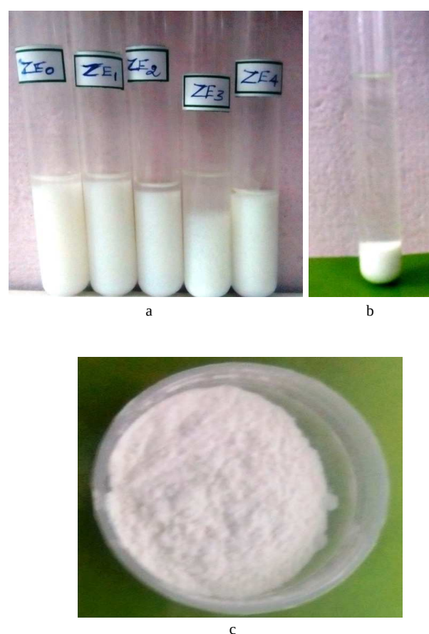
Fig. 2.4. The ZnO-NP preparation processes a) ZE0- Room temperature, ZE1-60°C, ZE2-70°C, ZE3- 80°C, ZE4- 90°C. b) Shows particles settle down c) Nanopowder
