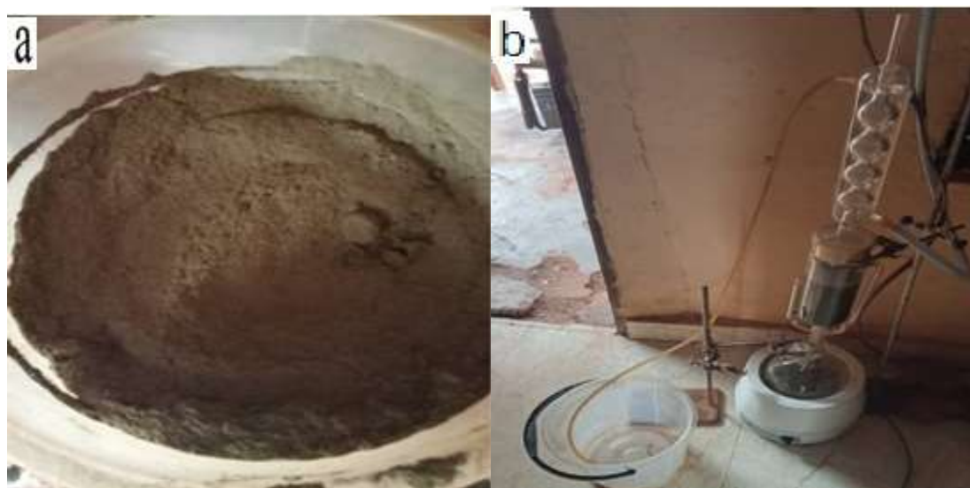
Fig 1.0: (a) Grounded powdered orange leaves and (b) Soxhlet extractor
