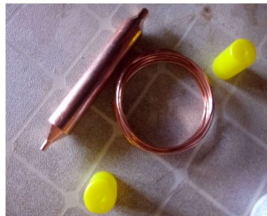
Fig.4 Desiccant dryer and capillary tube
