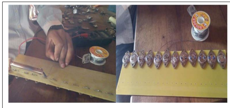
Figure 8: Assembling the transistor in series .
