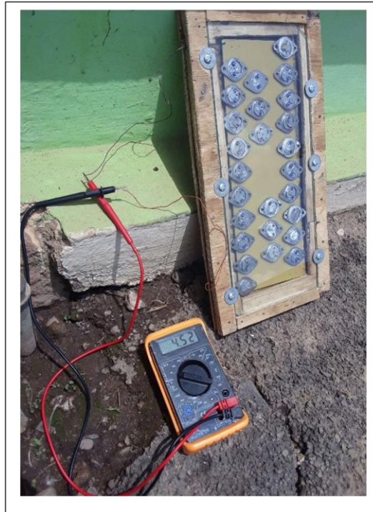
Figure 10: Voltage obtained by mounting the 13 transistors mounted in series .
