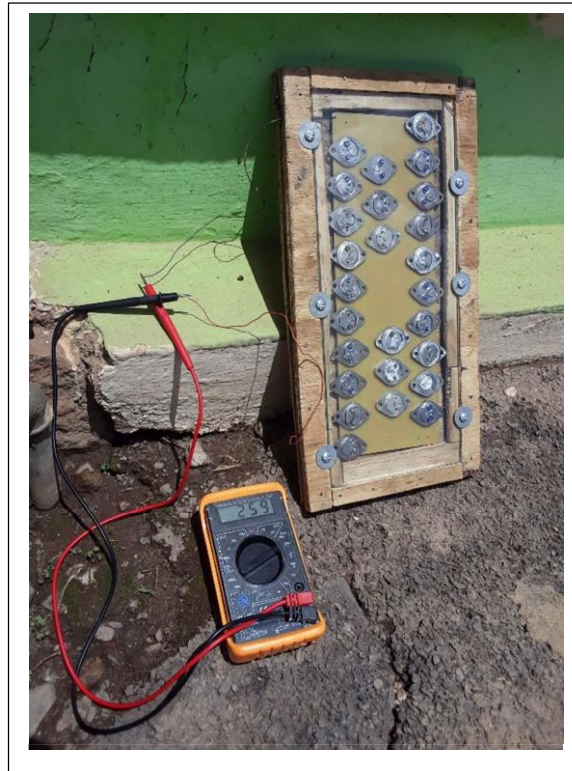
Figure 11: Current produced by the 13 transistors in series made in parallel with 13 other transistors in series .
