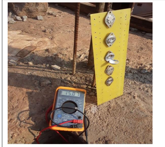
Figure 6: Voltage created by 5 transistors mounted in parallel
