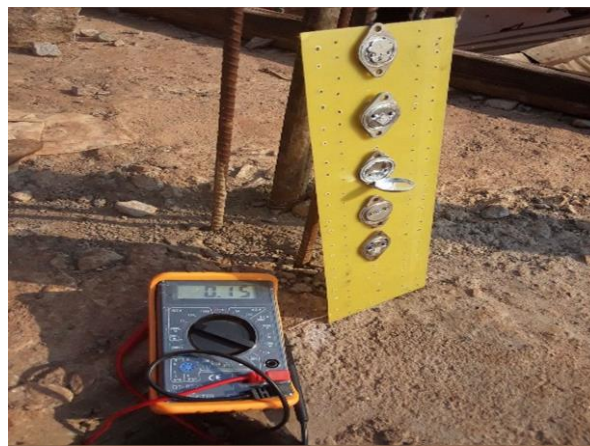
Figure 5: Current generated by 5 transistors connected in parallel.
