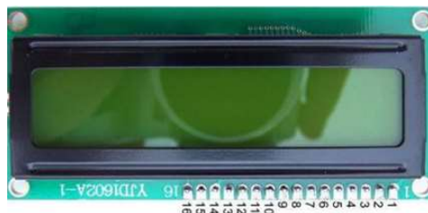
Figure 3: LCD display with 16 input pins.
