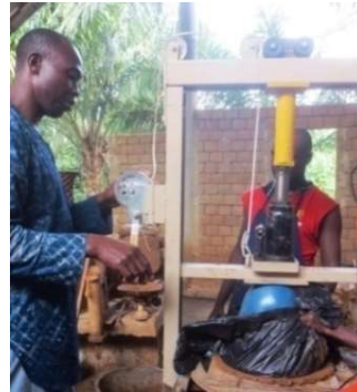
Plate 19 Hydraulic pressing metal mould for ceramic water filter at Atamora Pottery Studio
