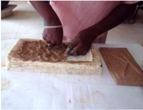
Plate 18 Casting of tile through pressing method in a plaster mould Photograph by Segun Abiodun Photograph by Damilola Oyewo
