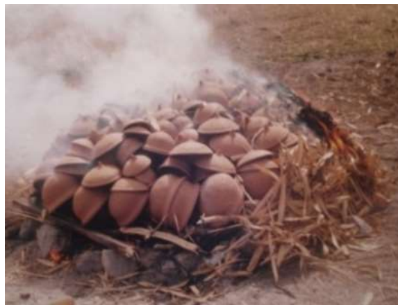
Plate 23 Yoruba indigenous open firing technique in Saki Photograph by Abokede Gbenga
