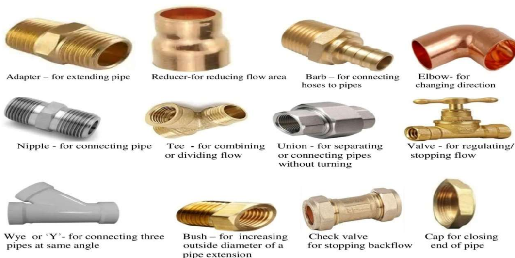
Figure 2 Common plumbing fittings
