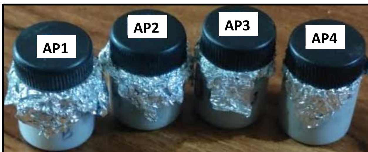
Figure 1. Four different sample holders (polyethylene bottles) containing experimental specimens of AP1, AP2, AP3, and AP4 cements are securely stoppered with aluminum foil layers internally.
