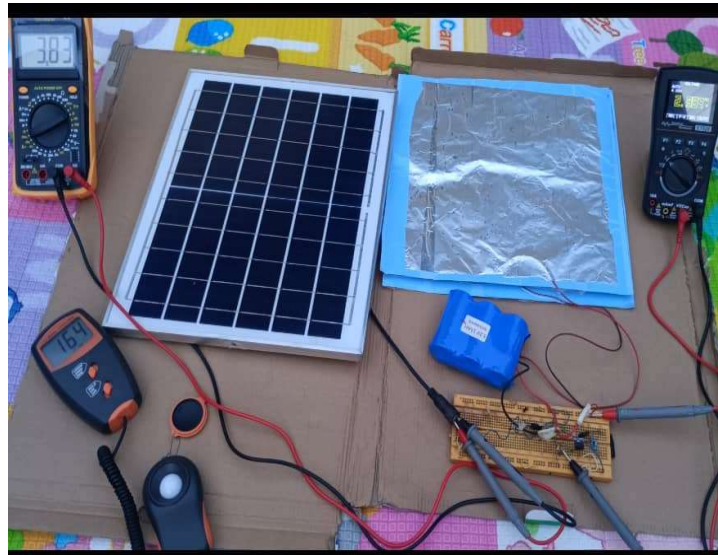
Fig 4. An Experimental setup for a hybridized PV and TENG. Size: 435x356x25
