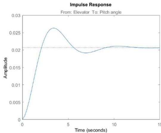
Figure 3 - Open loop impulse response (Pitch Angle  $\theta$ ).
