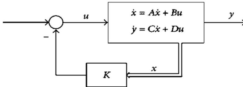
Figure 1 - Architecture of LQR control system.
