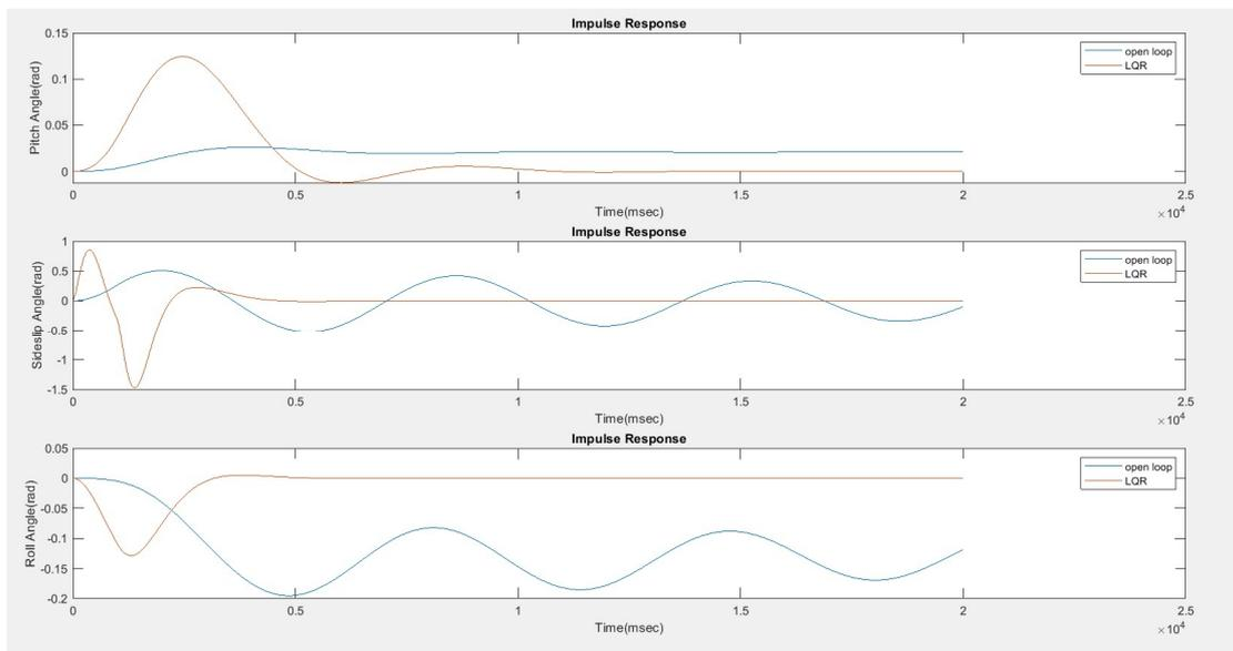
Figure 5 - Comparison of Open-loop and Closed-Loop Impulse Response
