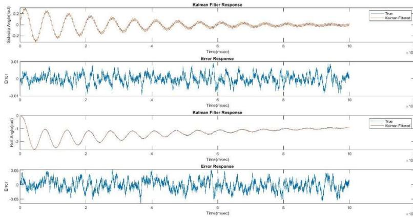
Figure 7 - Kalman Filter Response for the sideslip angle,  $\beta$  (b) Kalman Filter Response for the roll angle  $\phi$ .
