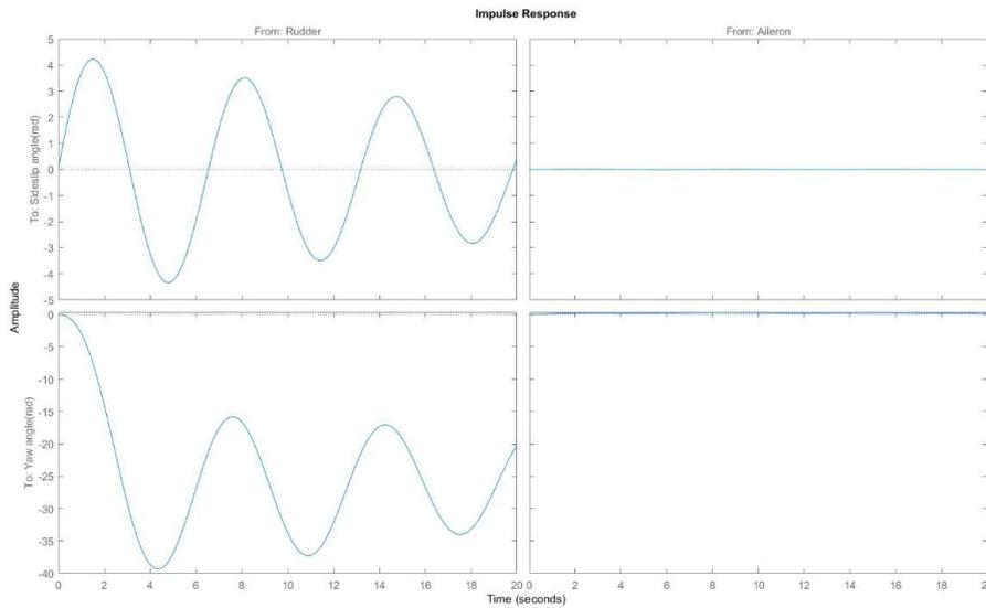
Figure 4 - Open loop impulse response (Sideslip Angle and Roll Angle)
