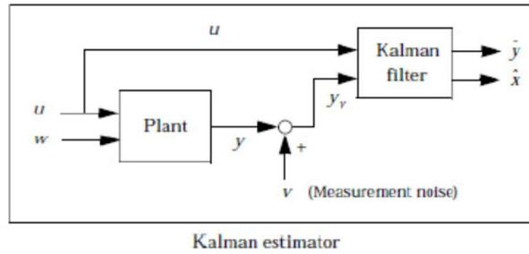
Figure 2 - Block representation of the Kalman estimator.
