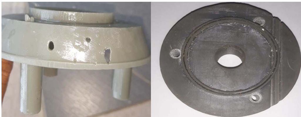
Picture 5. Failure on the outer surface and the inner surface
