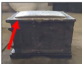
Figure 7. The surface of the concrete specimen experiences expansion as a result of the influence of aluminum slag.
