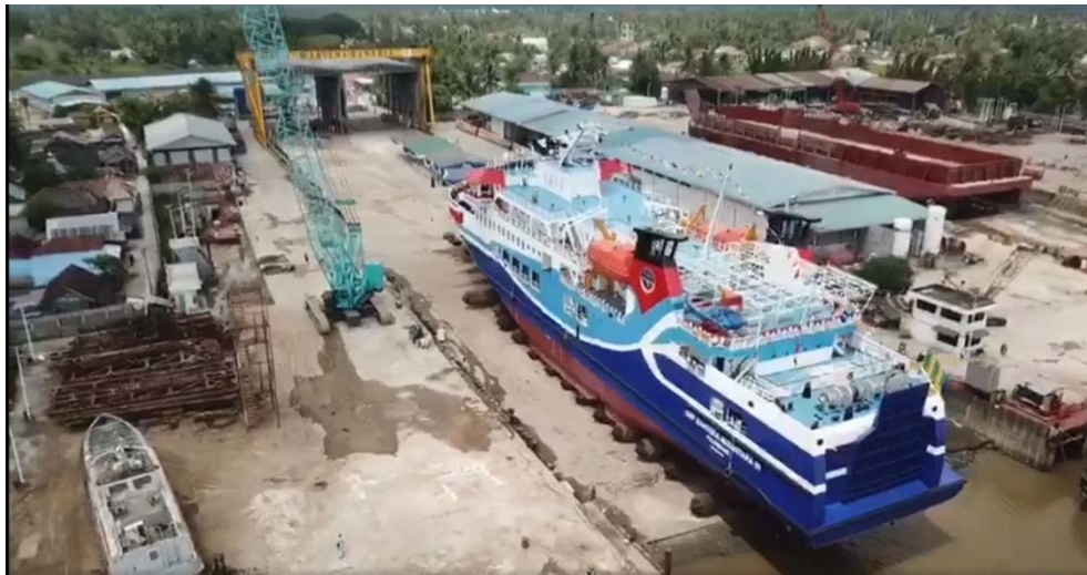
Figure 1 Launched of KMP Bahtera Nusantara 01, 1500-GT class Ro-Ro passenger ferry at PT. Mariana Bahagia Shipyard, Palembang
