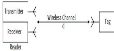
Fig. 1.4: The RFID system block diagram
