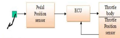
Fig 1.0 Block diagram of the ECU in a vehicle (Jyothi et al, 2012)
