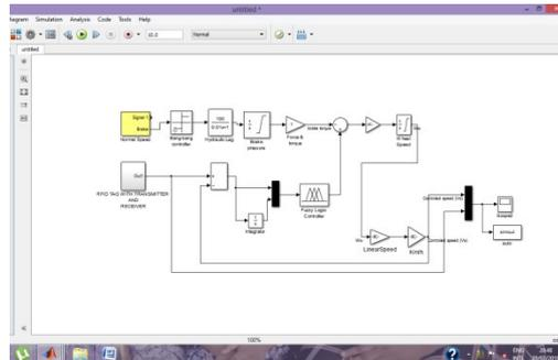
Fig. 1.3: Simulink model of the automatic vehicle speed control with RFID
