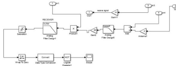
Fig 1.8: Simulink model of the RFID receiver.
