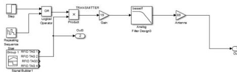
Figure 1.6: Simulink model of an RFID transmitter
