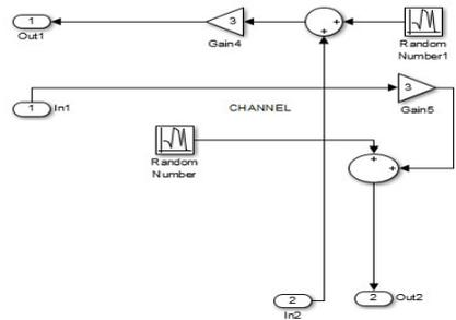
Fig. 1.7: Simulink channel modelling.
