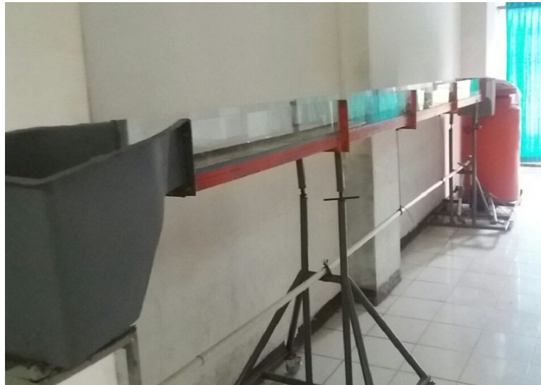
Figure 1. 2-Dimensional channel model (Syarifudin, A, 2018)
