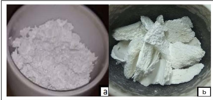
Fig. 2. CaO results in calcination of cow bones at a temperature of 1000 °C(a). For 6 hours (b). For 10 hours
