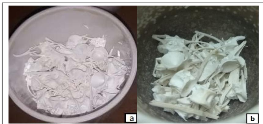
Fig. 3. CaO results from calcination of Tuna Bone at a temperature of 1000 °C(a). For 6 hours (b). For 10 hours
