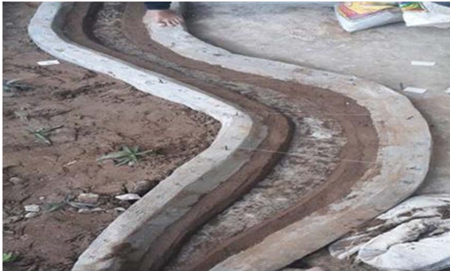
Fig. 2. Sketch of a river model in the Hydraulics Laboratory of Bina University Darma.(Achmad Syarifudin, 2018)
