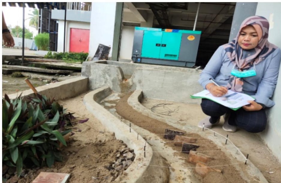
Fig. 2. Placement of the Cribs of 30° Slope Angle
