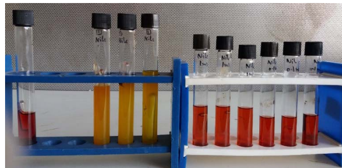
Fig (3): shown the presumptive test of the first Nile water sample After 48 h.
