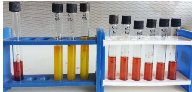
Fig (2): the presumptive test of the first Nile water sample After 24 h. The arrows show a change in the color of the nutrient medium in three test tubes that turned yellow with gas formation.
