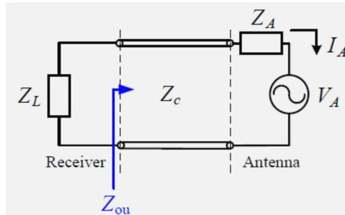
Fig 6: transmission line Thevenin equivalent circuit of a receiving antenna
