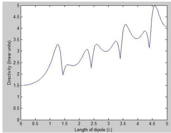
Fig 16: Peak directivity of the dipole antenna vs the length of the dipole
