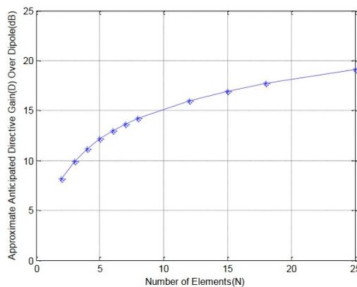
Fig 17: Graph of Directivity Gain versus Number of elements
