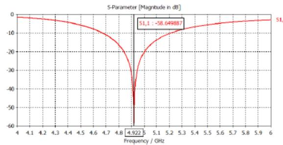
Fig 10: Return loss curve for the Half-wave dipole antenna.
