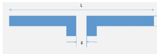
Fig 8: Half-wave dipole antenna
