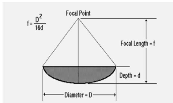
Fig 7: mathematical diagram of parabolic reflector
