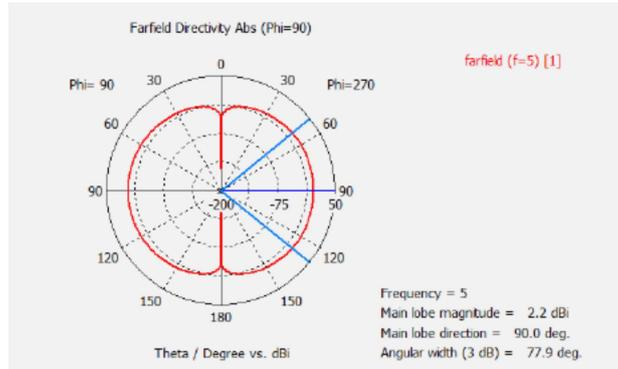
Fig 15: a polar plot for the elevation angle of the half-wave dipole antenna designed
