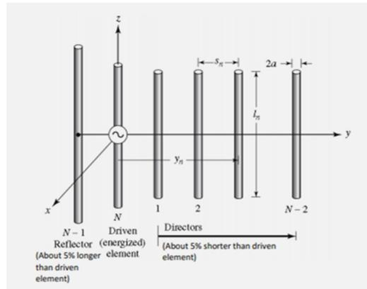
Fig 9: the elements of a Yagi antenna and their typical configuration.
