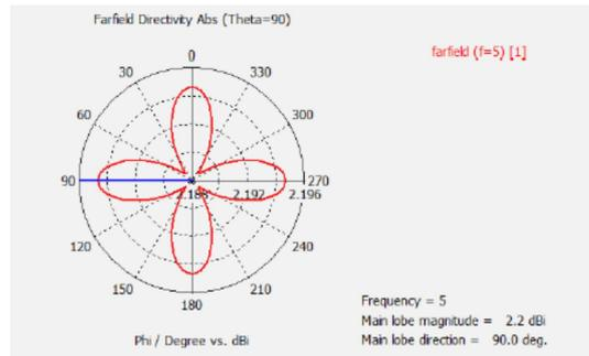
Fig 14: polar plot for Azimuthal Angle of the Designed half wave dipole antenna.
