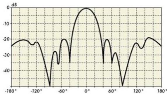
Fig 2: Antenna radiation pattern in Cartesian coordinate (rectangular form).
