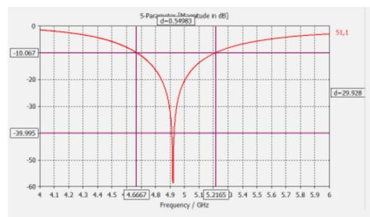
Fig 12: Bandwidth curve for the Half wave dipole antenna.
