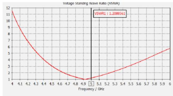
Fig 13: VSWR Plot of the designed half wave dipole antenna
