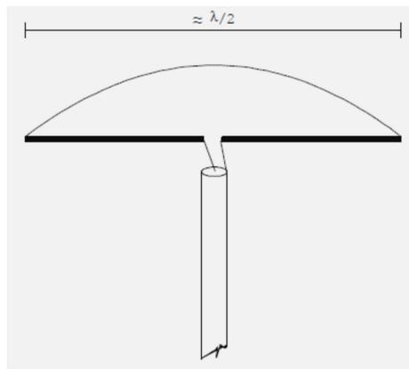
Fig 3: Tuned half-wave dipole
