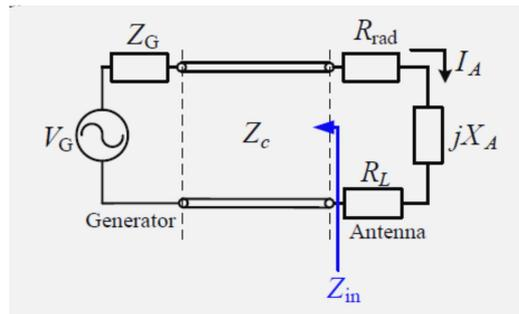
Fig 5: Transmission-line Thevenin equivalent circuit of a radiating (transmitting) antenna.
