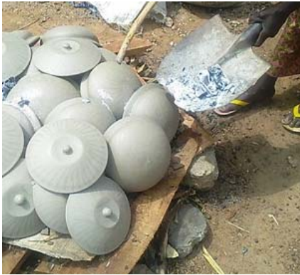
Plate 21. Introduction of embers in the kiln
