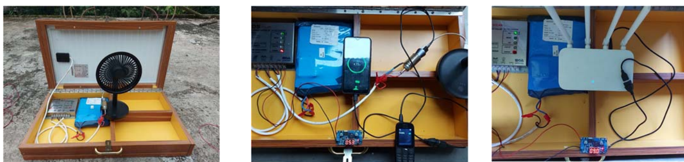
Fig. 3. Powering several devices at their required voltage; Powering fan (left); Charging smart phone at 12V and feature phone at 5.3V (middle); Powering router at 9V(right) [10]
