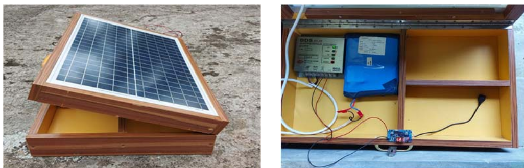
Fig. 2. External view (left) [10] and internal view with battery and controller (right) of Prototype
