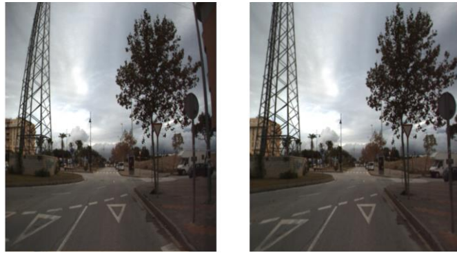
Figure 6: Image distorted by radial distortion (left) versus a perfectly perspective projected image(right).
