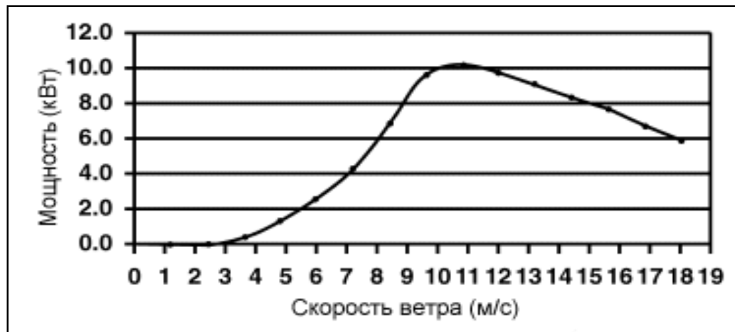
Figure 1. About the dependence of the rotor power on the wind speed
