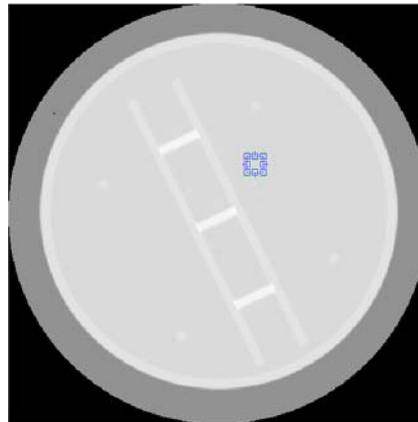
Fig. 2 Region of interest (ROI) location for noise and SNR measurements.
