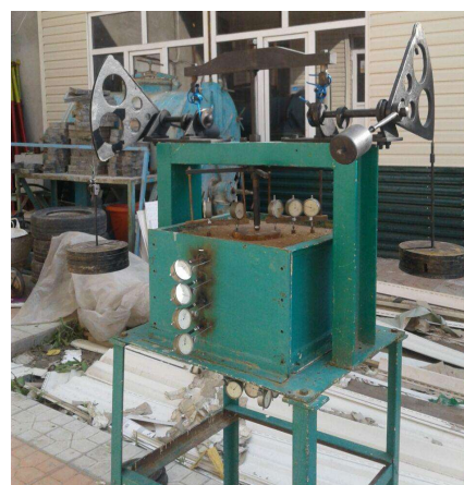
Fig-2. Bench scheme of indicators for measuring displacements, general view of the bench of measuring equipment: 1-volume tray with dimensions A \times B \times H = 45 \times 45 \times 30 \text{ cm}^3 ; 2-lower plate of the pressiometer; 3-upper plate of the pressiometer; 4-tared finely grained sand; 5 - coarse sand; 6-masses; h_I -V-horizontally directed indicators.
