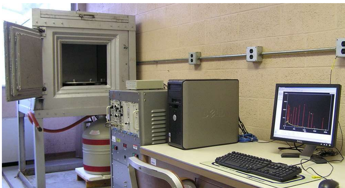
Fig.1: The Photograph Picture for High Pure Germanium Detector(HPGe) which used to Analyse the Samples.
