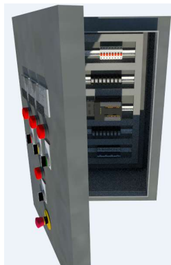
Figure 3.3.1.E. PLC position in the Panel
