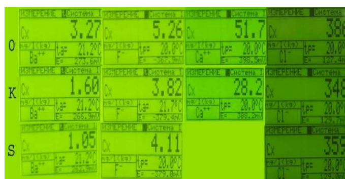
Figure 3. Quantitative indices of chemical components of initial and treated Borjomi mineral water in the condition of laminary regime of borehole – 37.
