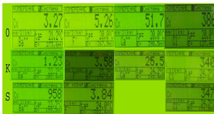
Figure 4. Quantitative indices of chemical components of initial and treated Borjomi mineral water in the conditions of turbulent regime of borehole 37
