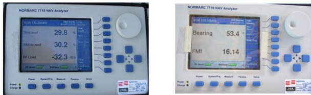
Fig 1. VOR parameters reading with Nav Analyzer
