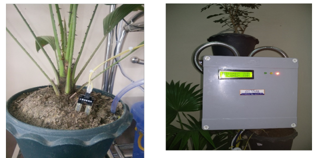
Figure-10 Sensing the Soil Moisture -Sensor 1
