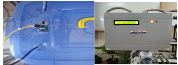
Figure-8 Water Level Testing condition (Stage 2 - Yellow LED)
