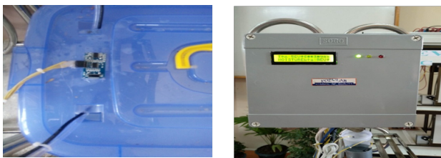
Figure-7 Water Level Testing condition (Stage 1 – Green LED)
