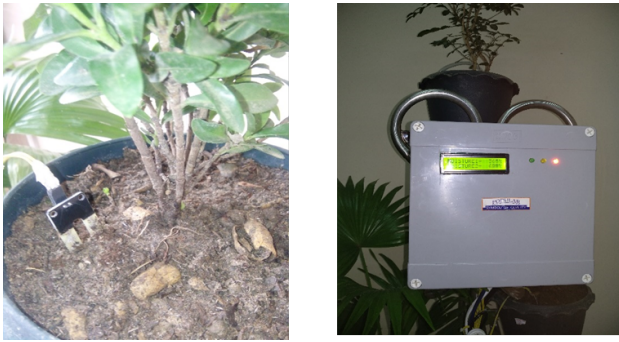
Figure-11 Sensing the Soil Moisture- Sensor 2
