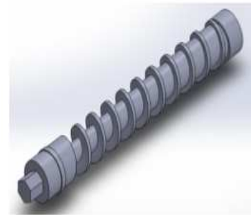
Figure 2. Modified Screw Shaft Design (15mm Pitch)
