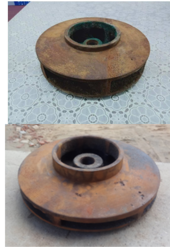
Fig. 4 Face width 18 mm Impeller and 12 mm Impeller
