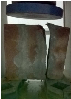
Figure 6: Fracture in one side
