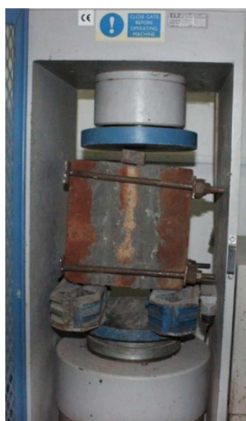
Figure 4: Triplet loading arrangement
